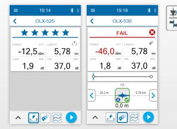
Figure 3. Optical Explorer displays power, length, loss and ORL in combined view.
