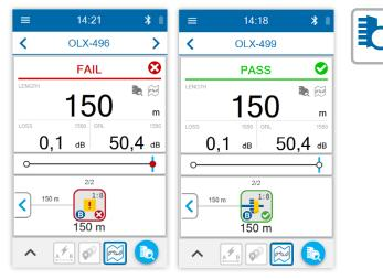
Figure 1. On the left, Optical Explorer informs the user that the expected splitter is not found. In second picture, Optical Explorer found the expected splitter, confirming link continuity.
